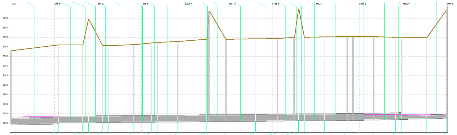
Hydraulic Profile: 2 nd Avenue South Parallel Tunnel, 10-year Level of Service
