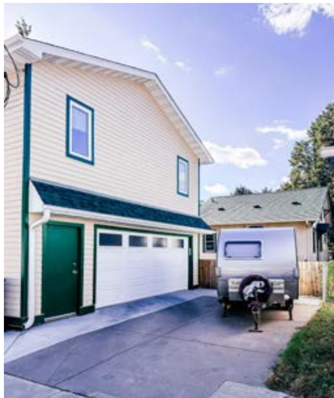
Although the zoning code only requires a garage door to be setback 5 feet from a side or rear lot line, more space may be needed for vehicle maneuvering. Most vehicles should have at least 17 to 20 feet of clear space to minimize turning movements from a garage to a public alley.
