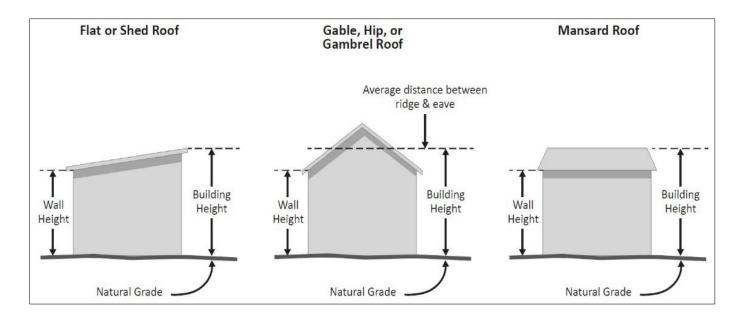
**HEIGHT:** Detached accessory structure height is measured from grade to the highest roof point of a shed/flat roof, the midpoint between the peak and the eaves for hip, gable, and gambrel roofs, and the deck level of a mansard roof.
