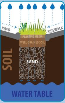
Green infrastructure slows down the flow of stormwater, allowing more runoff to infiltrate into the ground. This makes the water cycle in an urban environment closer to the natural water cycle.
