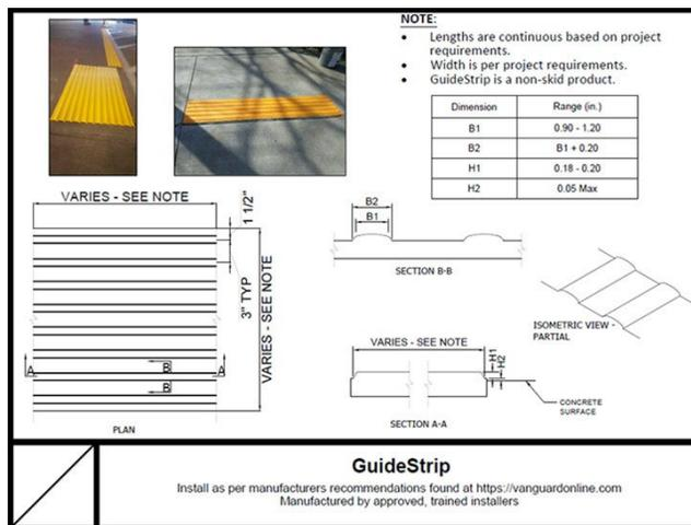
Figure 6: installation details for MMA tactile edge product from the manufacturer, Vanguard
