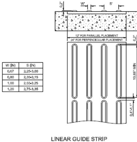
Figure 3: tactile edge standard plate used for the Hennepin Ave and 4<sup>th</sup> St reconstruction projects
