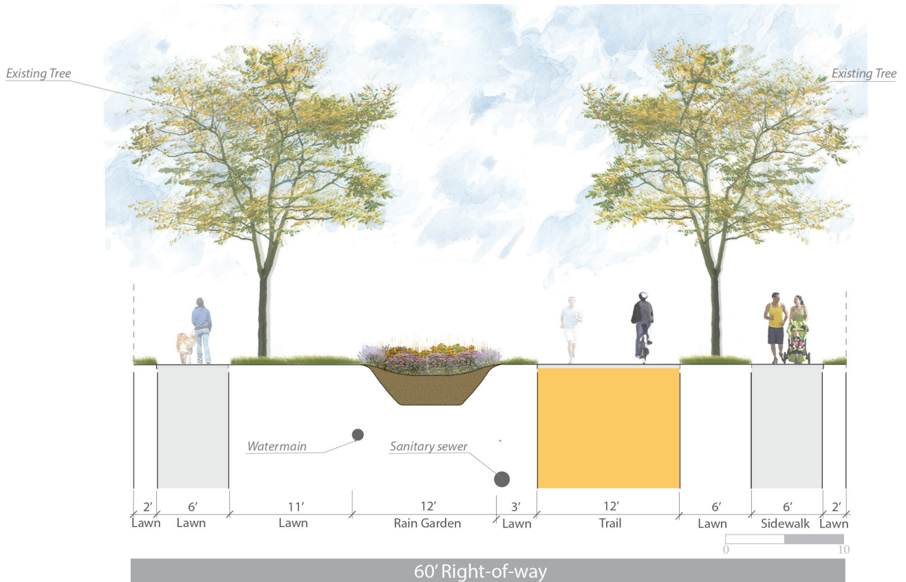
FIGURE 26 SHALLOW RAIN GARDENS (OPTION A): SECTION
