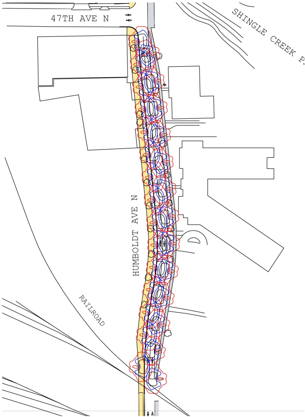
FIGURE 21 LIGHTING ANALYSIS: HALF AND HALF, TWO-WAY
