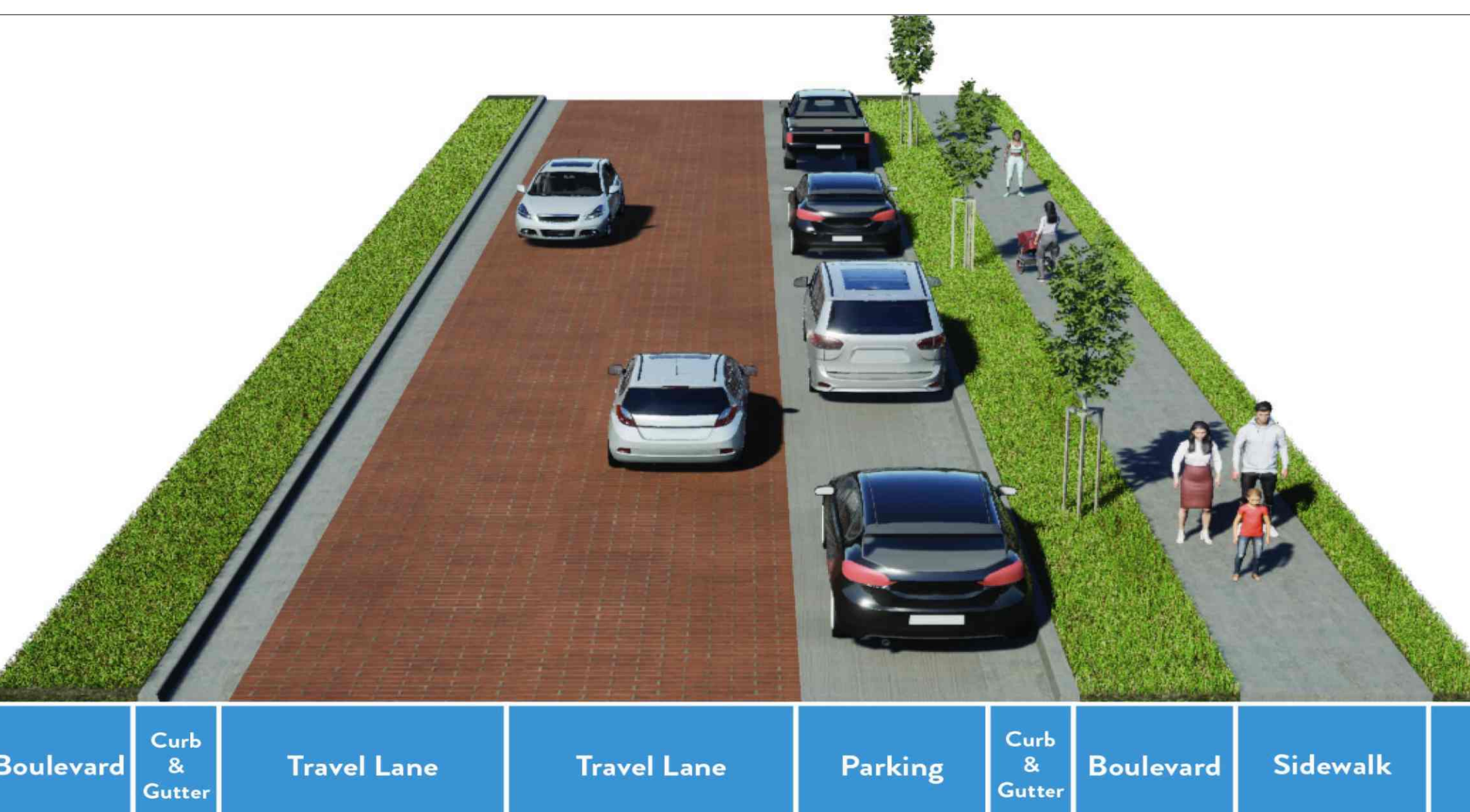
TYPICAL SECTION D-D QUINCY ST NE (SOUTH)
