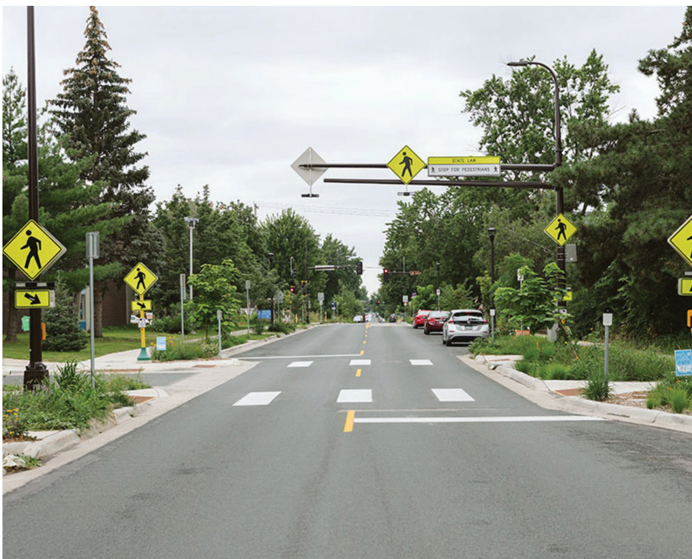
Rapid flashing beacon
