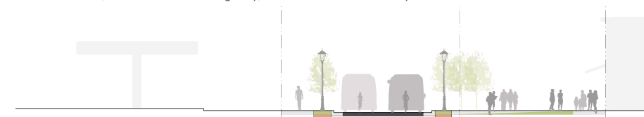
Limited Access Framework Section A-A Chicago Avenue (Looking North) Pedestrian, bicycle and transit mall, with access for emergency, maintenance and delivery vehicles.
