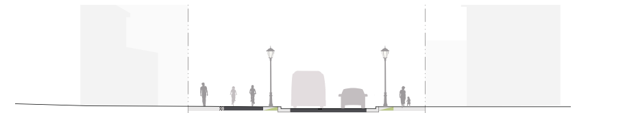
Typical Section B-B 38th St (Looking West) Section west of GFS, will be refined to integrate into existing network and the intersection at Chicago Ave.
