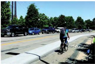
Illustrative rendering of curb protected bikeway–the City has installed this treatment on Oak St.
