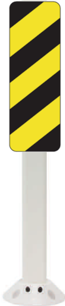
6" x 18" OM3-R Sign, mounted to 39" white flexible delineator. Plastic, retroreflective
