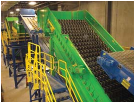
Improved screens, optical sorters and front end metering
